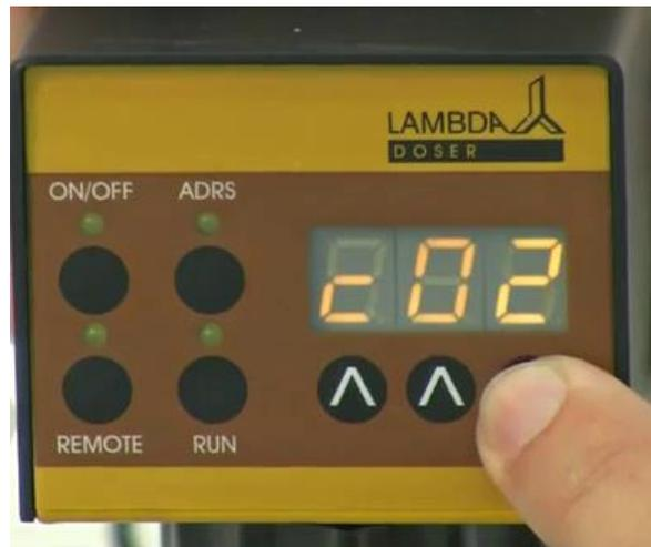
**Figure 2-14:** If the same program has to be repeated twice, increase the cycle number to “**c02**” by pressing the buttons  $\wedge \wedge \wedge$  below the display (from 0 to 99 cycles). The program can be repeated up to 99 times, indicated by “**c99**”. If 0 is entered for the cycle number “**c00**”, the program will run continuously (**infinite loop**).
