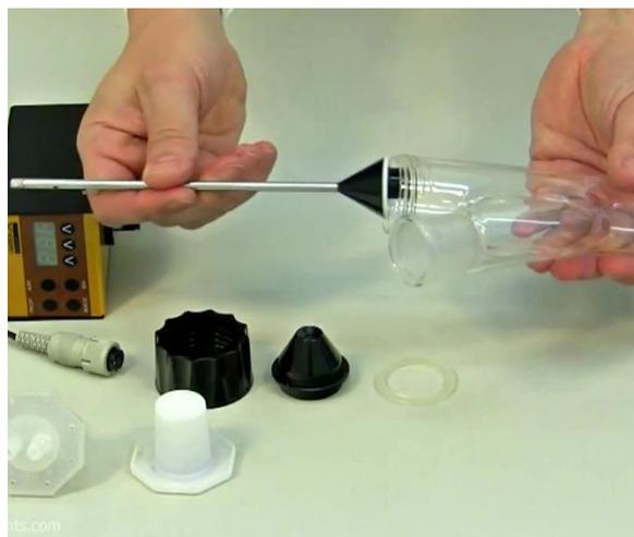
**Figure 1-4:** Insert the distributor (standard) inside the ~0.2 l glass vessel with its opening directed downwards so that it will not be damaged.
