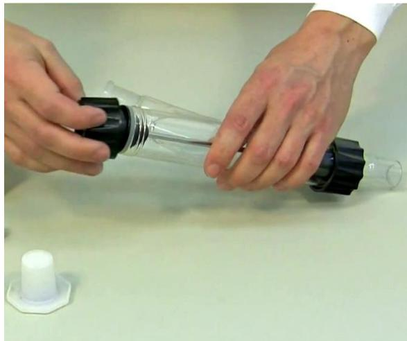
**Figure 1-8:** Secure the centering part with the rubber seal through the axis of the distributor with the screw cap to the glass vessel.
