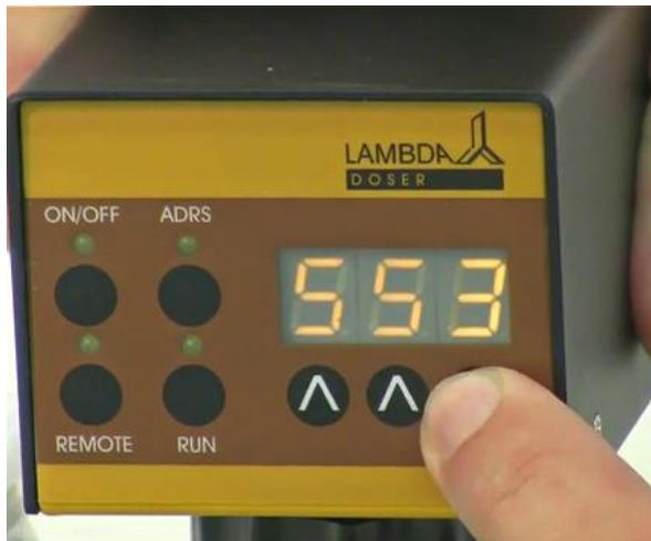
**Figure 1-13:** Choosing the speed of powder addition with the help of control buttons **^ ^ ^**.
