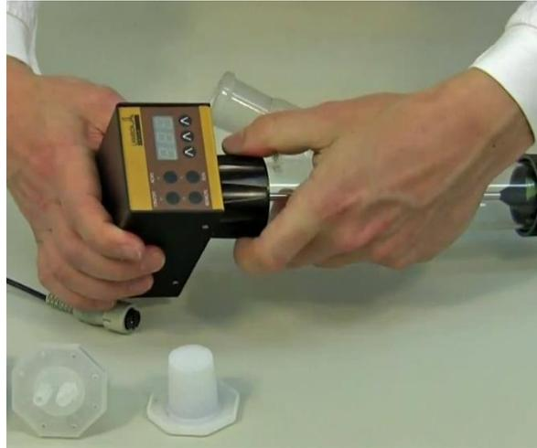
**Figure 1-10:** Press the axis of the motor unit completely inside the centering part. So that, the metal pin of the motor unit will fit into one of the six corresponding holes in the centering unit. This assures a perfect seal of the DOSER and a sufficient pressure of the distributor against the teflon disc in the bottom of the Doser vessel.
