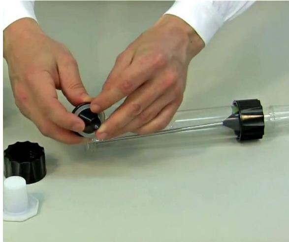
**Figure 1-6:** Place the tefflon treated rubber seal on the centering part with the tefflon layer facing outside (towards the glass vessel).
