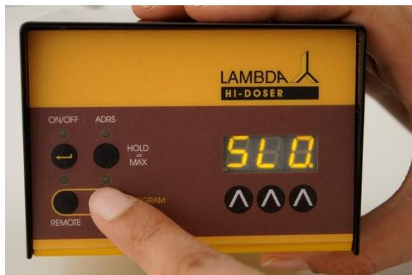
**Figure 1-16** Press the **RUN** button, to select the desired speed mode (**FAS / SLO**). Confirm and save the chosen speed mode by pressing the **ON/OFF** button on the control panel.
