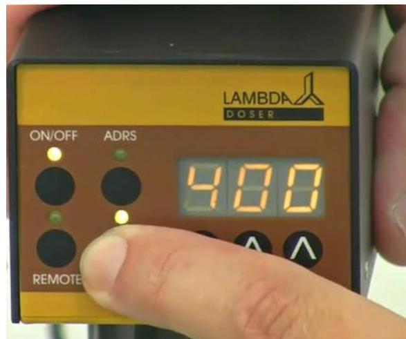
**Figure 2-16:** To **START** the program, press the **RUN** button. The **RUN** and **ON/OFF** LEDs are on.
