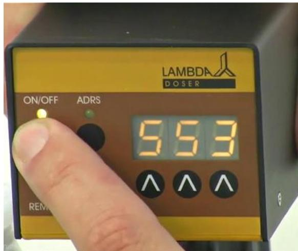
**Figure 1-14:** Pressing ON/OFF button on the DOSER motor unit after choosing the dosing speed.
