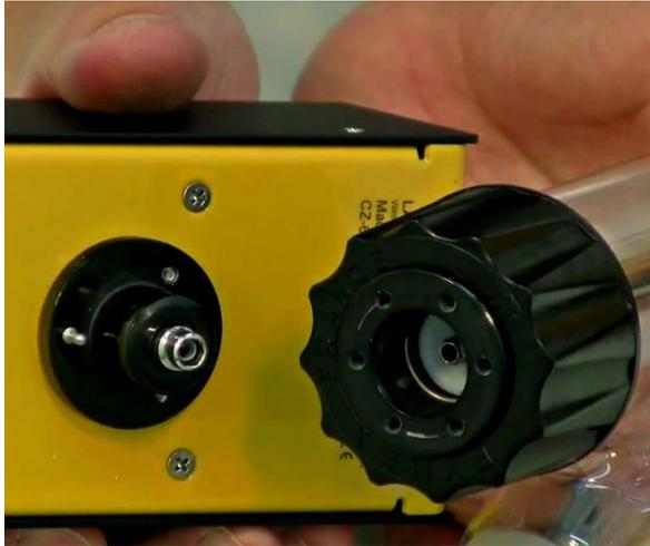
**Figure 1-9:** Axis of the motor unit with metal pins and the centering part with six holes.
