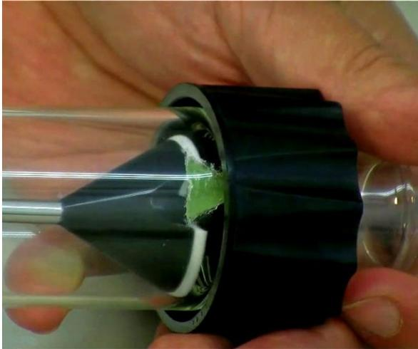
**Figure 1-5:** A silicon baffle/scraper can be found on the lowest part of the glass vessel. The distributor must be turned with its opening towards the baffle/scraper.
