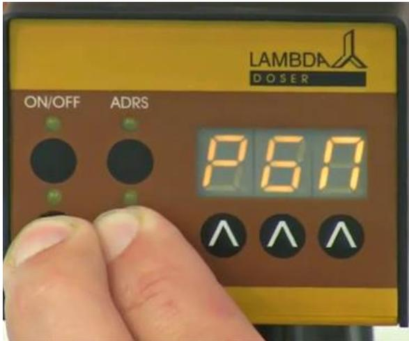
**Figure 2-1:** Pressing Remote and Run buttons simultaneously and the "**PGM**" indication appears.
