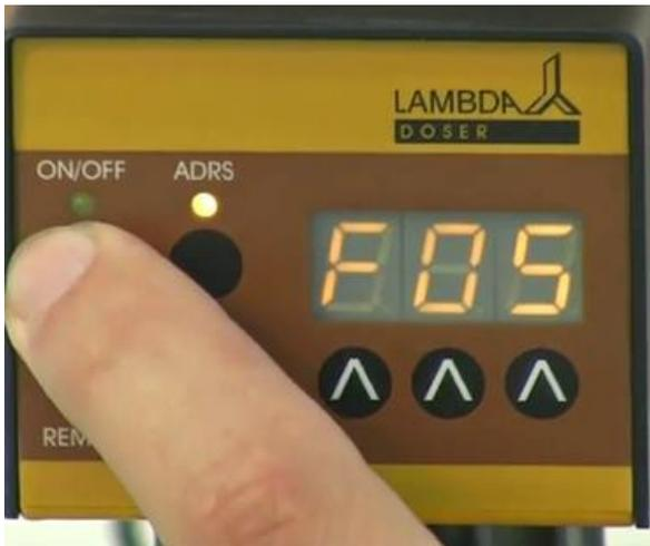
**Figure 2-11:** After having entered the time of the last step, press the **ON/OFF** button. The flow rate (000) of the next step which will not be programmed appears on the display. For example: “F05”
