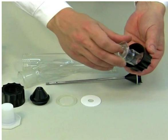
**Figure 1-1:** Insert the ground glass piece through the threaded screw cap SVL 42.
