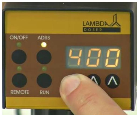
**Figure 2-4:** Set the desired flow rate value for the first program step by pressing the buttons **AAA** below the display (from 0 to 999, corresponding to 0 to 100% of the motor rotation speed).
