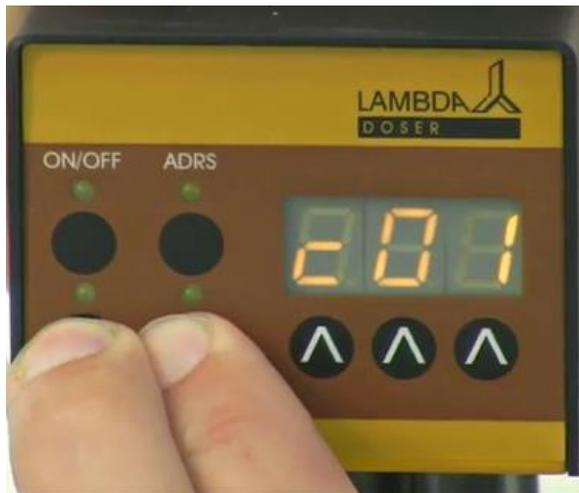
**Figure 2-13:** Press both **REMOTE** and **RUN** buttons simultaneously and the indication “**c01**” will appear on the display. This indicates that the program will be executed only once and the powder dosing instrument will stop afterwards.
