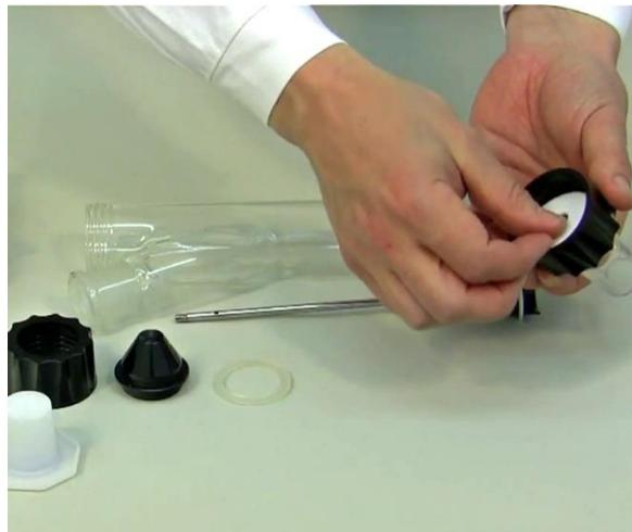
**Figure 1-2:** Place the teflon disc inside the screw cap on the top of ground glass piece (NS 29/32).
