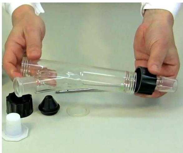
**Figure 1-3:** Screw and secure the ~0.2 l glass vessel to the screw cap with the teflon disc and ground glass piece.
